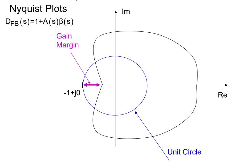
Gain margin is 1 – magnitude of A $\beta$  when the angle of A $\beta$  =180°
