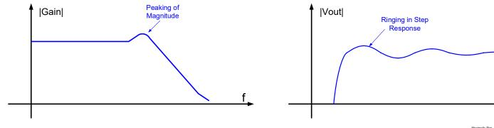
45° pole-pair angle corresponds to  $Q = \frac{1}{\sqrt{2}}$ 90° pole angle (on pole pair) corresponds to  $Q = \frac{1}{2}$
